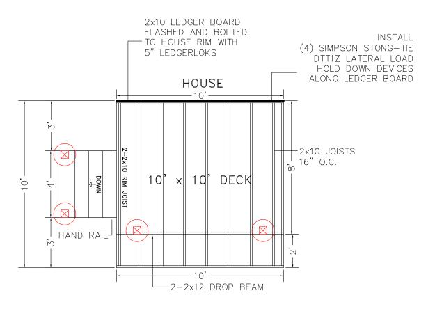
2x10 LEDGER BOARD FLASHED AND BOLTED TO HOUSE RIM WITH 5" LEDGERLOKS JOISTS TO BE 2x10 SYP TREATED INSTALLED 16" O.C.
